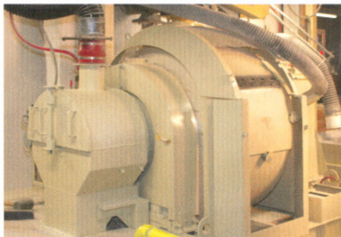
The rotary batch mixer features a horizontal, rotating drum with a stationary inlet at one end and a stationary outlet at the other.
